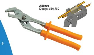
Looking for simplify the work of the electrician, in applying the wedge connectors KARA and KARA T family, KRJ developed the **ALIKARA**. With an angle of handhold differentiated and adapted teeth, making the operation easiest and allows extraction of connector, without an extra conventional extractor needs. Made only in the version of 12" inch (30cm minimum length), thickness 8mm head and 1kV insulation. Perfect tool for application of all sorts of wedge connector family KARA and KARA T.
